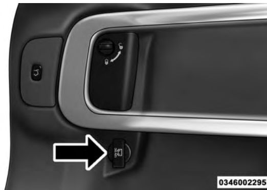
Rear Electrical Power Outlet
